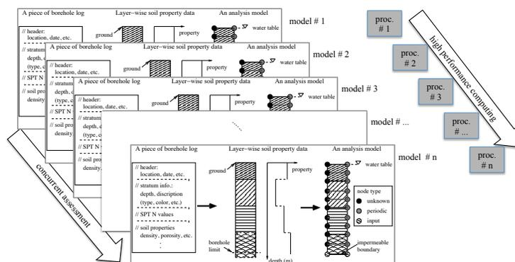
Figure 16.8: Multiple models constructed for numerical experiment of uncertainty estimation of liquefaction
