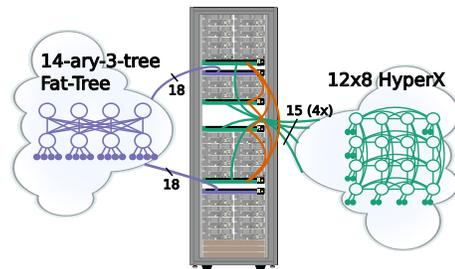
Figure 15.4: Depiction of one of 24 racks of our 672-node supercomputer with two edge switches connecting to the 3-level Fat-Tree and four switches for the 12x8 HyperX network (brown = rack-internal passive copper cables; gaps used for cable management)
