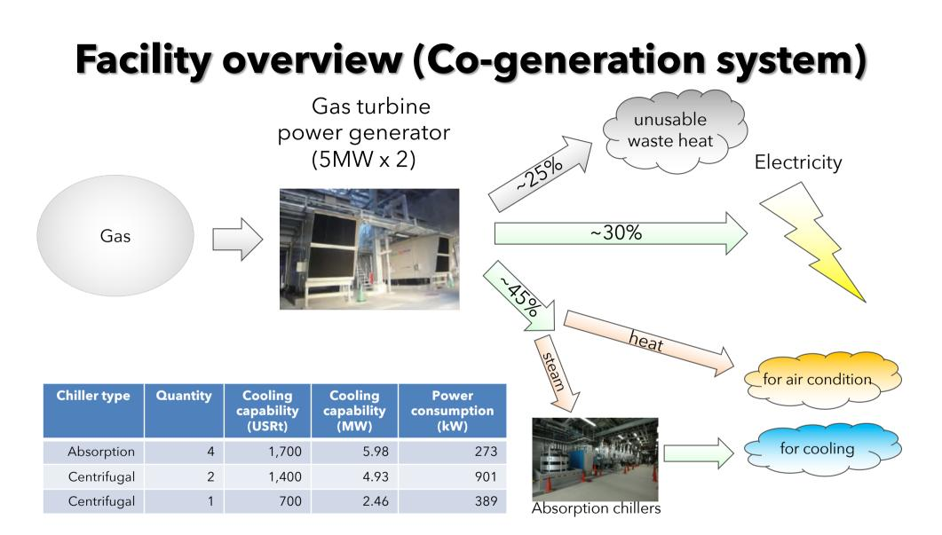
Co-generation system enables to achieve higher energy efficiency On the other hand, due to tight connection between power generator and chiller, facility operation is much more complicated.
