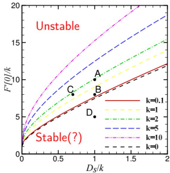
Fig. 2: Neutral curves for different  $k$ . The upper side of the curve is the instability regime.
