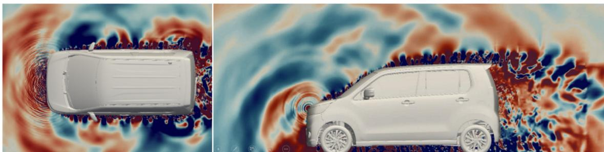
Figure 13.5: The propagation of the Pressure fluctuation.
