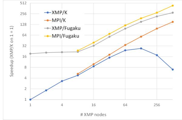
Figure 2.2: Speedup of CCS QCD on Fugaku and Performance comparing to the K computer
