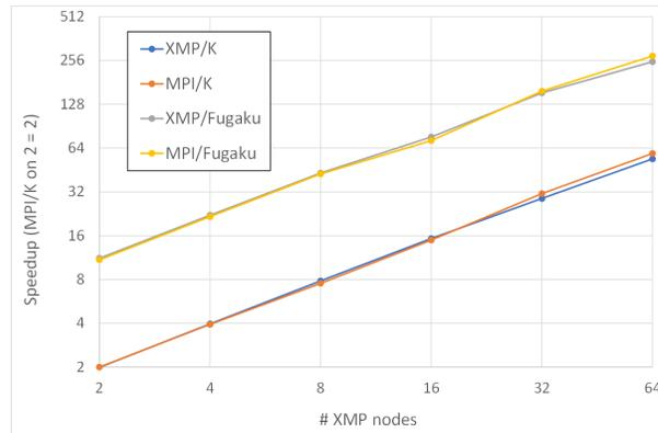
Figure 2.3: Speedup of NTChem-MINI on Fugaku and Performance comparing to the K computer
