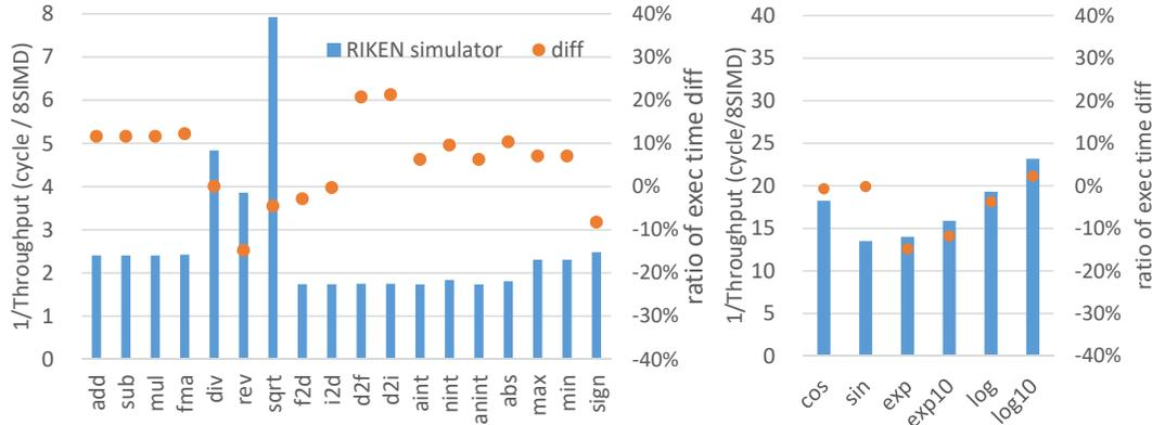
Figure 2.4: Execution throughput of kernel benchmark (double precision) in the RIKEN simulator and the execution time difference ratio of the test chip
