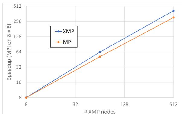
Figure 2.1: Speedup of Impact3D on Fugaku and Performance comparing to K computer
