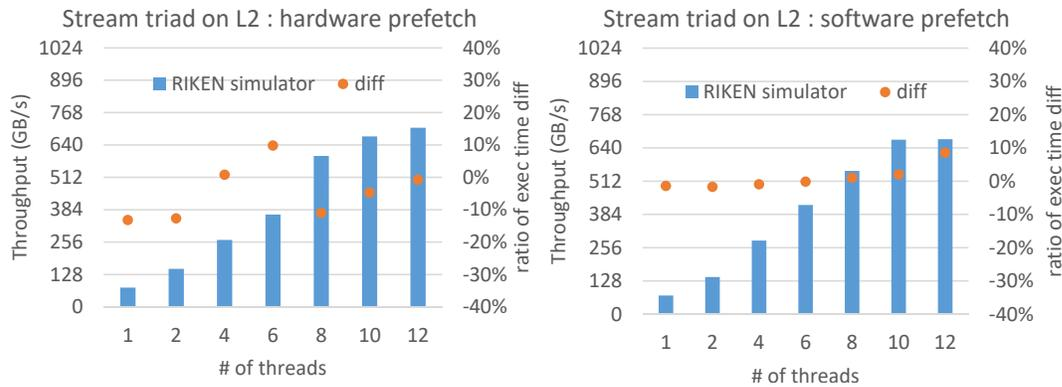
Figure 2.5: L2 cache throughput of Stream Triad in the RIKEN simulator and the difference in execution time with the test chip
