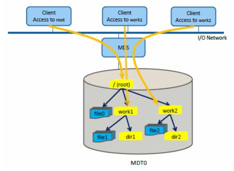
In a single MDS configuration, metadata for the entire file system is managed by a single MDS/MDT pair, so metadata access becomes a performance bottleneck as the size of the file system increases. In a multi-MDS configuration, metadata can be managed by multiple MDS/
