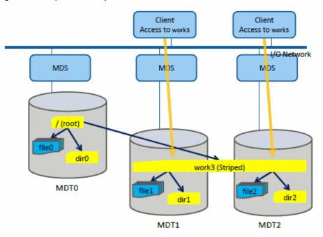
In the above example, the metadata of directories dir1 and dir2 and files file1 and file2 under /work3 are distributed and stored in MDT1 and MDT2, respectively.
