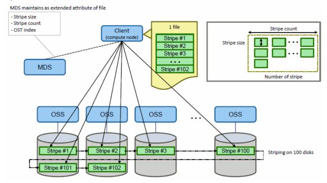
With the lfs setstripe command, you can specify a size and range for the data to be distributed, and the number of units of data to be distributed.
