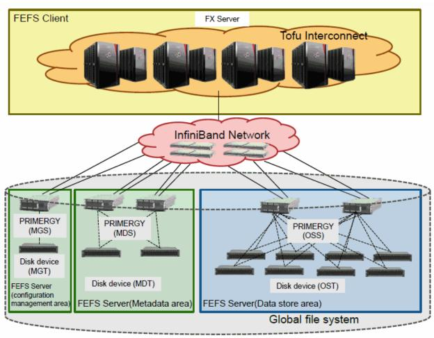
Figure 1.1 Hardware configuration using FX server
