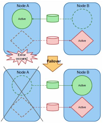
Figure 2.12 Active/Standby failover configuration
