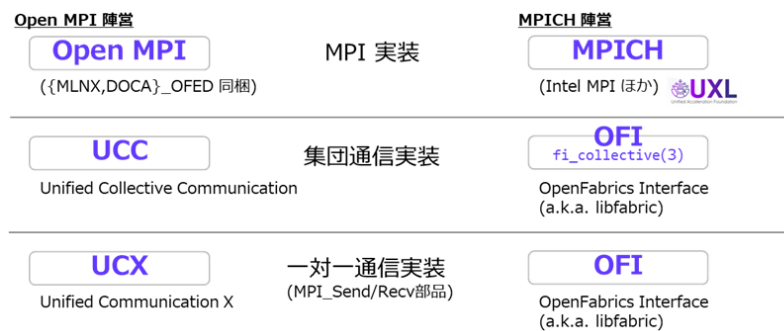
Figure3-21 Implementation comparison of the communication layers of Open MPI and MPICH
