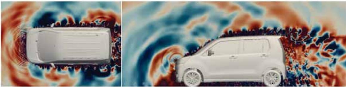
Figure 13.5: The propagation of the Pressure fluctuation.
