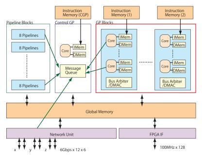
Fig. 2. Block diagram of MDGRAPE-4 SoC.
