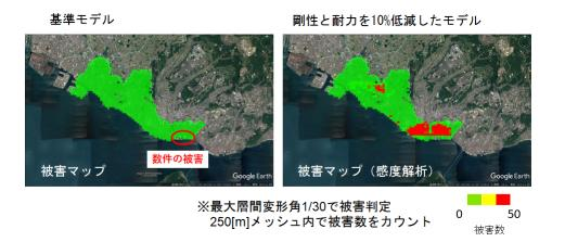
Figure 16.3: Comparison of degree and distribution of earthquake damage of residential buildings by using normal and weak analysis models
