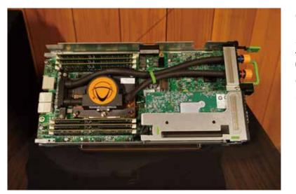
Computation node (Fujitsu PRIMERGY) with single chip Intel Xeon Phi 7250 (Knights Landing, 68 cores, 3+ TFLOPS) and Intel Omni-Path Architecture card (100Gbps)
