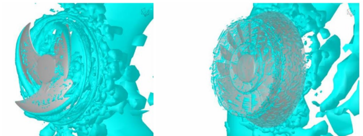
Fig. 2: Comparison of vortex structures around blades for the current fan (left) and improved fan (right)
