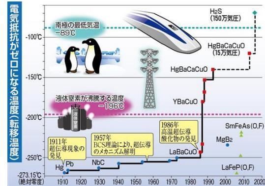
Superconducting transition temperature
